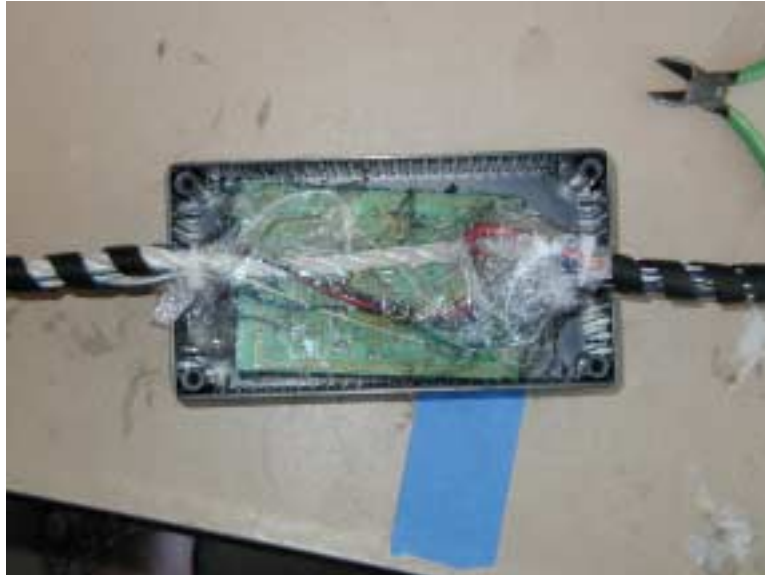
Figure 14 Encasing the circuit board
