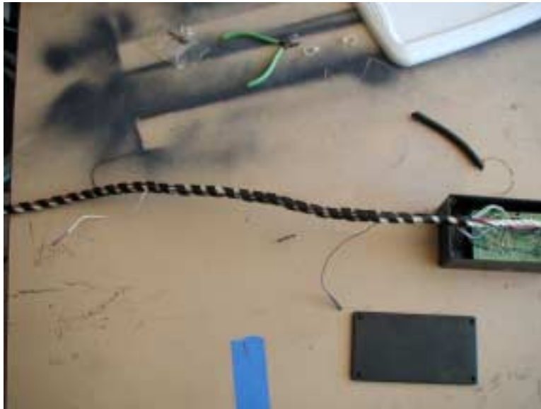
Figure 13 Wrapping the wires with coil wrap
